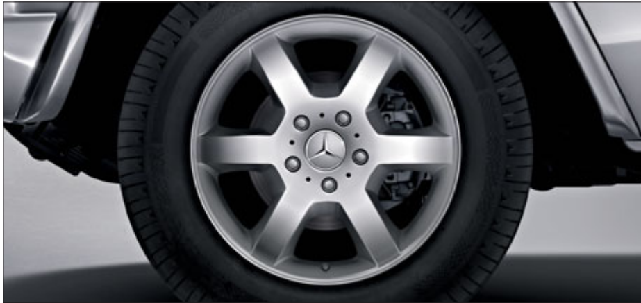
6-spoke light-alloy wheels with 265/60 R 18 tyres, with high-shine finish (option for G 350 BlueTEC, G 500, Code RL6)
