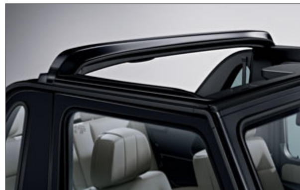
The roll-over bar makes open-top driving a safe pleasure
